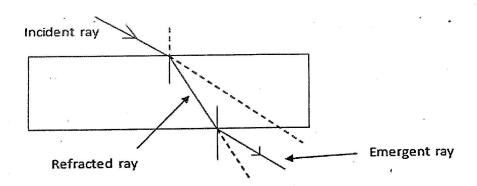
iii) The change in angle of light ray is the same when it enters and leaves the glass. The direction of incident ray is parallel to the direction of emergent ray. The two rays are parallel.
