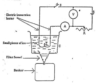
b) Describe how you would use the apparatus above to determine the specific latent heat of fusion of ice.
